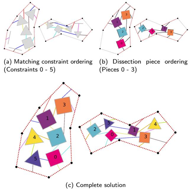
Fig. 14. Two different partial solutions (a), (b) which lead to the same complete solution (c). Ordering by matching constraint means that all the boundary intervals in the partial solution have connections. Ordering by dissection piece means that the connectivity of several boundary intervals (dashed lines) is unknown. In (a) boundary interval connections are colored by matching constraint.
