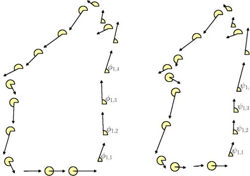
Fig. 16. Visualizing the angular optimization problem. Vector magnitudes are ignored and we optimize only over vector angles. The notation is shown for some of the angles ( $\phi$  and  $\psi$ ) used in the optimization problem.
