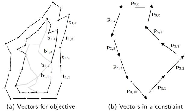
Fig. 10. (a) Edge vectors involved in the objective function for Equation 1. (b) Edge vectors involved in the constraint for a piece in Equation 1.
